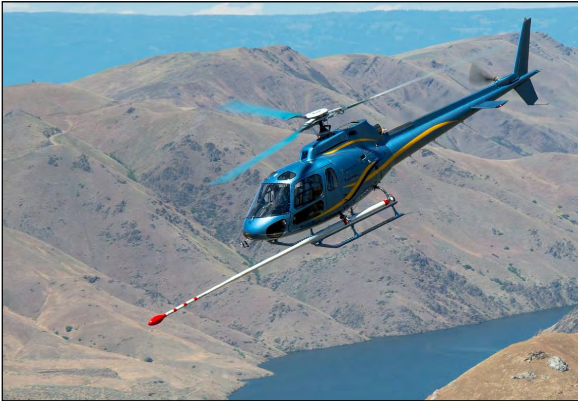
Figure 11: Eurocopter AS350 helicopter is equipped with mag stinger for magnetic data acquisition, and internal spectrometer crystals for radiometric data acquisition.
