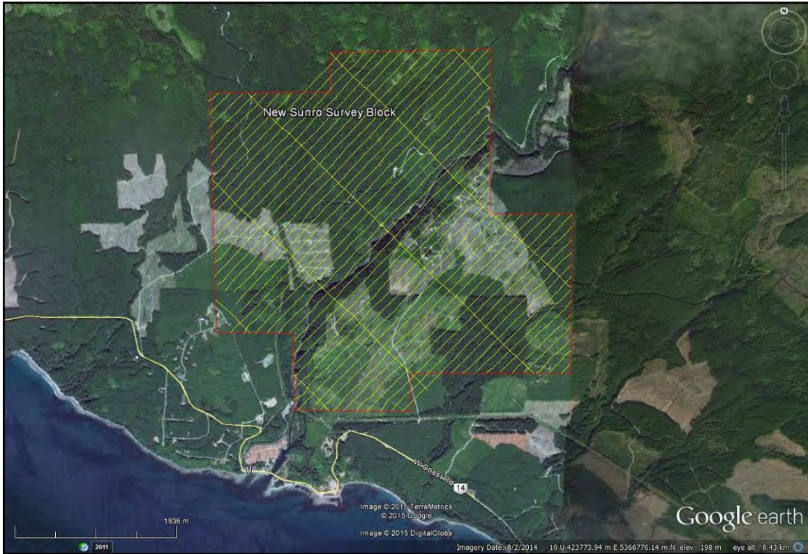
Figure 3: Plan View –New Sunro survey block boundary in red with flight lines displayed in yellow.
