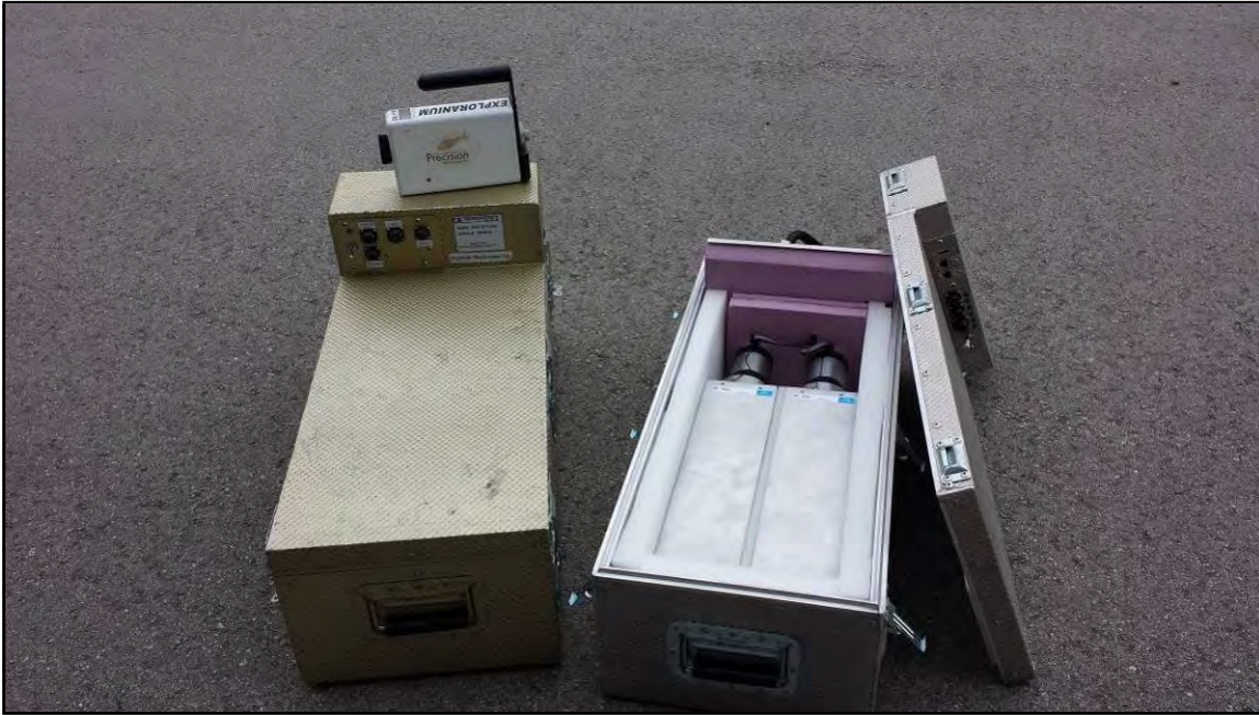
Figure 14: GRS-10 Thallium-activated Sodium Iodide spectrometer crystal pack. The open unit on the right shows two individual 4.2 liter detectors.
