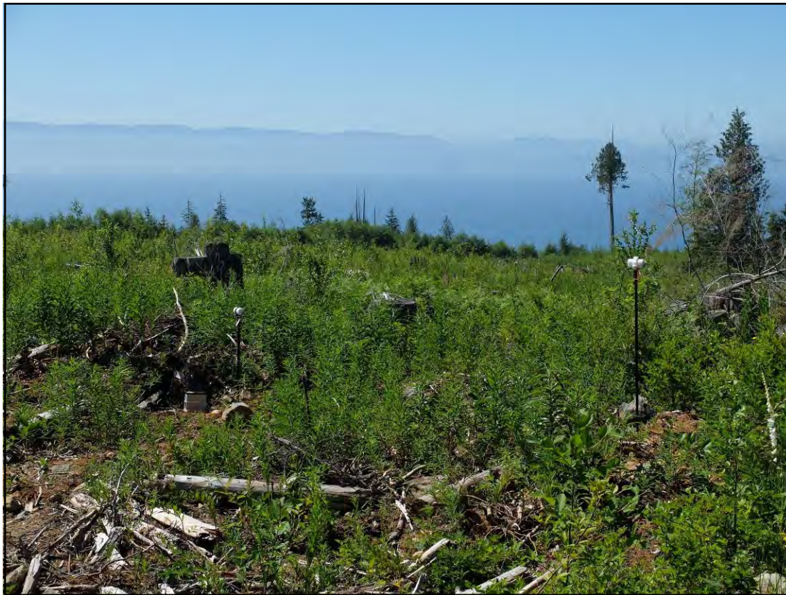
Figure 7: GEM 1 (left) and GEM 4 (right) magnetic base stations located within the survey block.
