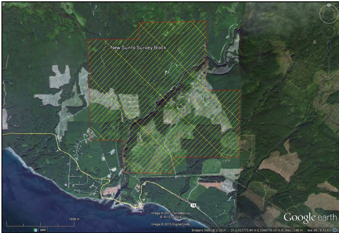
Figure 3: Plan View –New Sunro survey block boundary in red with flight lines displayed in yellow.
